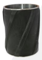
The rubber centralizer is an essential downhole tool accessory used in drilling, cementing, and well completion operations. During the running-in process, it utilizes the supportive force of rubber blades to counteract the casing's self-weight and lateral pressure from the wellbore wall, keeping the casing centered in the wellbore and ultimately enhancing cementing quality and wellbore sealing integrity.
