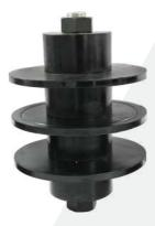
The wiper plug / drill pipe dart is a rubber sealing component used in drilling operations to isolate drilling fluid inside the drill pipe from cement slurry (or workover fluid), preventing internal fluid migration within the drill pipe. Installed in the inner groove of the drill pipe joint, it achieves sealing at the tool joint through elastic deformation of the rubber.
